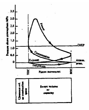
Figure Indicator diagram
