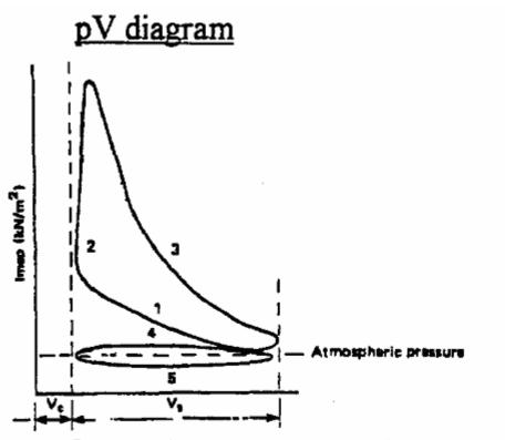
Fig. Pressure-volume indicator diagram. (1) compression, (2) combustion, (3) expansion, (4) exhaust, (5) induction.
