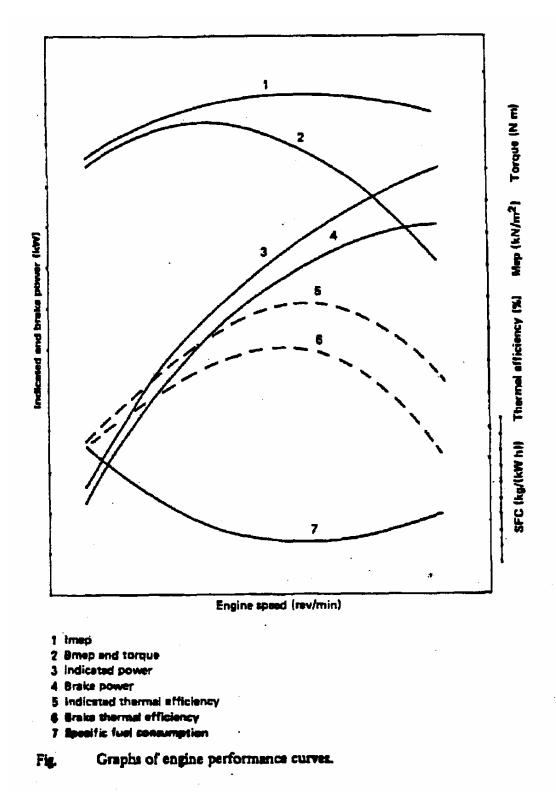
bmep = imep  $\eta_m$  $\eta_{th i} = \frac{P_i}{(kg/h) CV}$  Factors affect the engine torque and power:
