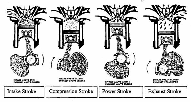
\* <u>Intake (induction or inlet) stroke</u>: The intake valve has opened. The piston is moving downward, drawing a mixture of air and gasoline vapor into the cylinder. \* <u>Compression stroke</u>: The intake valve has closed. The piston is moving upward, compressing the mixture.
