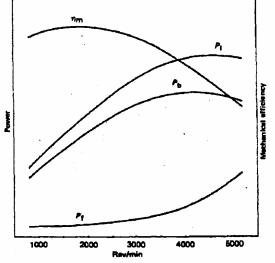
Fig. Indicated power  $(P_i)$ , brake power  $(P_b)$ , mechanical efficiency  $(\eta_m)$  and frictional power  $(P_f)$  plotted on a rev/min base.
