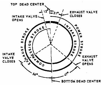
Fig Intake- and exhaust-valve timing. The complete cycle of events is shown as a 720° spiral, which represents two complete crankshaft revolutions. Timing of valves different engines.
