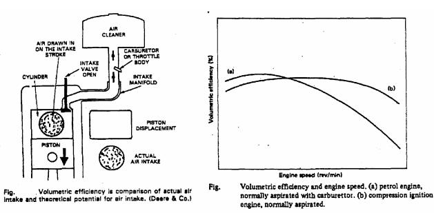
\* Volumetric efficiency depends upon throttle opening and engine speed as well as induction and exhaust system layout, port size and valve timing and opening duration.
